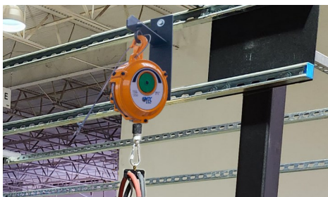
BCR-H5-KIT Hanging Cable Balancer w/MOUNT-BCR-H5
