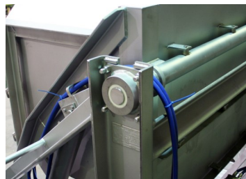
Nylon Pivot Bearings in Stainless-Steel Housing; 3" Dia Solid Pivot Shaft
