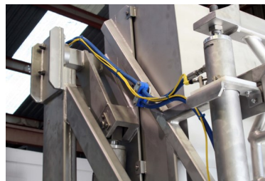
Raising of BNB Hold-Down controlled by Photo Sensors
