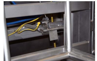
Container Load-In Controlled by Photo Sensors
