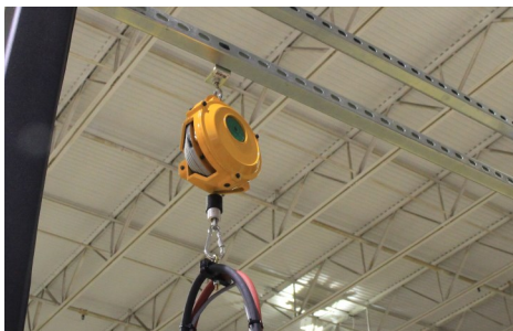
BCR-H5-KIT Hanging Cable Balancer
