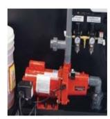
The MWTS Recycle System includes a pressure pump that is set to turn off at pressure above 50 PSI and turn on at lower pressure. Pumps are fully automated and do not require a pressure tank to maintain pressure.
