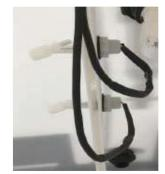
Liquid Level Sensors: Reed Type Liquid Level Sensors are used throughout the system to monitor the water levels in the tanks. Liquid Level Sensors control the flow of water into and out of the surge tank.
