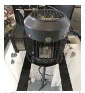
The Paddle Mixer in the treatment tank turns on when the top liquid Level sensor in the treatment tank has lifted. The mixer motor speed is controlled by a VFD (Variable Frequency Drive) and is preset to 25 Hz.
