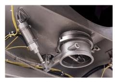
Air-operated liquid drain.
