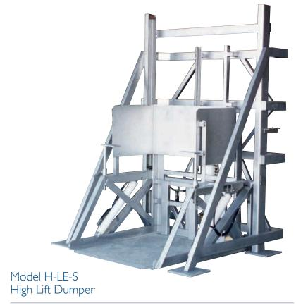
The standard design of the H-LE-S is an all tube and channel construction with minimal floor contact for easy sanitation. It features the same design as the H-LE High Lift Dumper except for the straight stationary frame.
