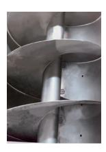
The stainless steel screw continuously moves product through the Continuous Cooker.
