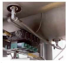
Quick disconnect direct steam injector.
