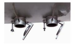
Low velocity steam injectors with quick opening cover for sanitation.
