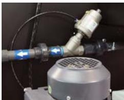
The MWTS utilizes an air-operated stainless steel slant valve as it performs well in environments with debris and corrosive materials.
