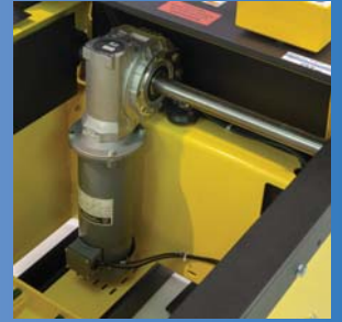
Electric Gearmotor drives two roller chains, moving the battery in and out of the carriage
